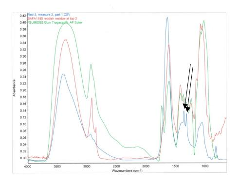
Note for example the two sharp peaks in the "fingerprint region" of the spectrum from the intact bottle that are not present in either the gum tragacanth reference spectrum or in the reddish residue from the Kiribati bottle.
