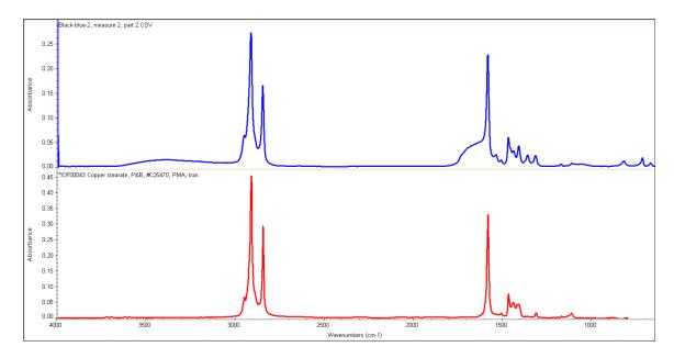
The cap data from EAG was also analyzed using Winterthur's protocols and databases, and again we reach the same conclusion as EAG – the material is cellulose, and as such may represent a fragment of a paper liner from the interior of the cap. See Figure 2 below.
