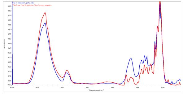
The reddish residue identified both in the non-archaeological bottle and in Kiribati fragment 2-8-s-2a was found to be cellulosic in nature (predominately based on the O-H stretching band  $\sim 3500~\rm cm^{-1}$  and the bands between 1050 and 1100 cm<sup>-1</sup>, as well as the carbonyl band  $\sim 1700~\rm cm^{-1}$  and several other bands in the fingerprint region between 1500
