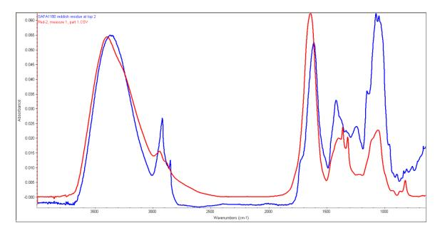
Similarly, the brown residue in the bottom of the bottle appears to be cellulosic in nature (see Figure 4 below).
