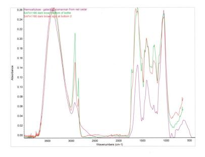
Figure 7, shown below, reveals a favorable comparison between gum Arabic and the reddish residue in the Kiribati bottle. However, FTIR is insufficient to distinguish between different types of plant gums, and gas chromatography-mass spectrometry is necessary to definitively distinguish between gum tragacanth and gum Arabic.
