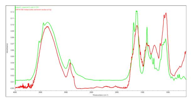
There are additional bands in the sample from the intact bottle that are not in the cellulose reference spectrum, however, suggesting that there may be an additional component in the Kiribati sample beyond a plant gum such as gum tragacanth (see Figure 5 below).
